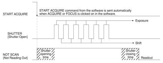
Figure 43. Free Run Timing Diagram
